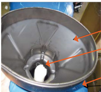
Fig. E Use a suitable funnel for pouring the media into the tank
