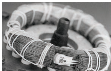
Fig. 46 Thermal switch incorporated in windings
