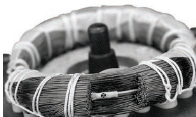
Fig. 44 PTC sensor incorporated in windings
